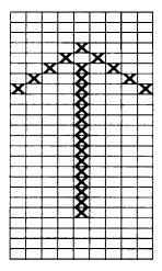
Now you translate the dot pattern you've created on paper to a numeric format so you can send the information to your printer. Every dot has an assigned value. Each vertical column (which has a maximum of **24** dots) is first divided into three groups of eight dots. Each group of eight dots is represented by one byte. Since one byte consists of eight bits, one bit represents one dot.
